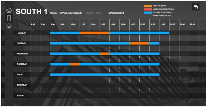
Fig. 7. Screenshot of the HVAC schedule which provides a visualisation of the operation time of the HVAC as a function of the occupancy of the rooms
