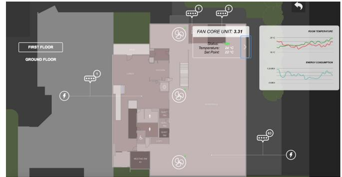
Fig. 4. Screenshot of the building view, it provides a link to the energy and comfort dashboard for each room. It also displays the position and status of the HVAC assets. By clicking on an asset, the user can display specific information (Status, Inside temperature and Set Points in the case of HVAC)
