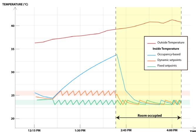
Fig. 9. Impact of the HVAC strategy on the inside temperature in function of the outside temperature. The blue curve represents an occupancy-based strategy, the orange one the dynamic setpoints strategy and the green one the fixed setpoints strategy.
