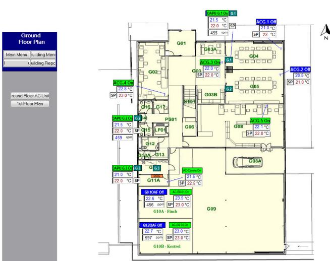
Fig. 1. Screenshot of the current BMS system of the university. This page provides monitoring information regarding the AC units of a building using a map-based visualisation.
